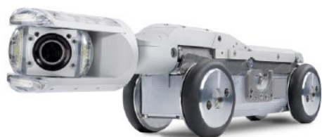
A CCTV camera is used to capture images of Cambridge's storm sewers.
