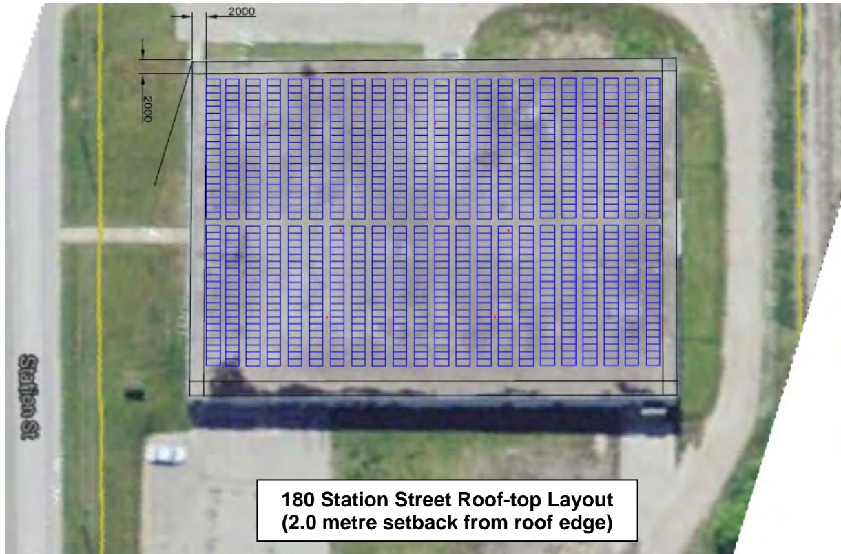
Figure 2 Example of Roof-top Solar Install & Layout for 180 Station Street
